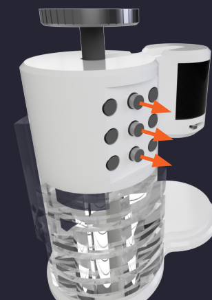
figure 15: Control panel with nine generic dials that retract when not coupled to a function.
