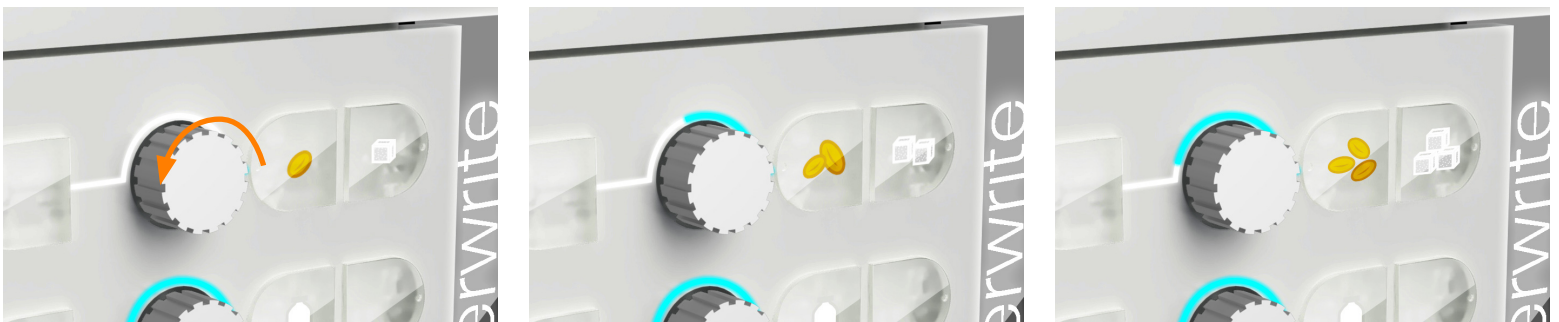
figure 26: The progression of augmented feedback from the LED ring and icons shows the value of each parameter.
